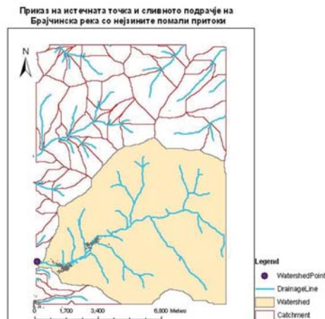
Fig.3 Layout of the outlet point at the gauging station with the upstream watershed area.
